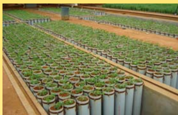
Picture 3: High throughput lysimetric setup, allowing the weighing of approximately 500-600 lysimeters/day, with 5 workers. It allows accurate assessment of water uptake in a large range of materials. Current capacity: 2400 cylinders
