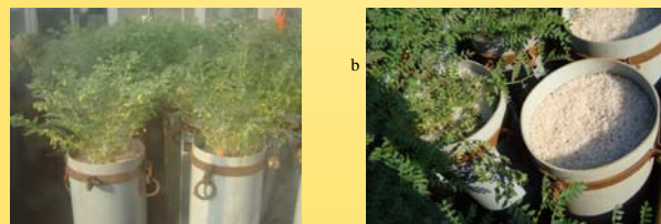
Pictures 2 a & b: Chickpea growing in the lysimeters under receding moisture (left), in which pods can be seen and polyethylene beads covering the surface of the cylinder to prevent evaporation (right)
