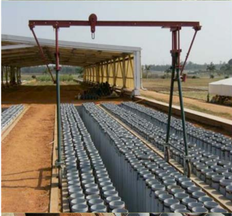
Crane for lifting root cylinders for moisture under water stress determinations
