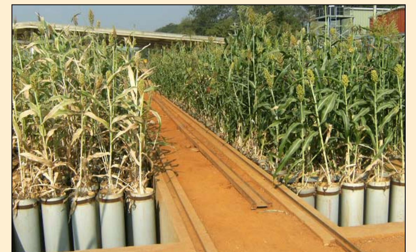
Fig. 3. Lysimetric study of sorghum variation for water extraction (WE) and transpiration efficiency (TE) under post-flowering drought stress.
