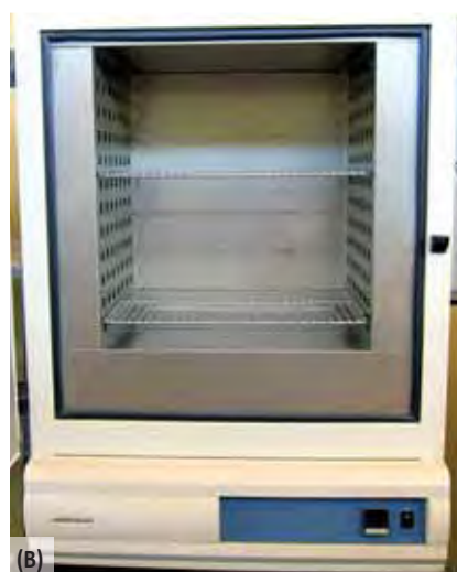
Figure 22.1. Drying ovens: (A) large capacity forced-draft oven; and, (B) small capacity non-draft oven (suitable for drying open container samples; e.g., soil moisture samples).
