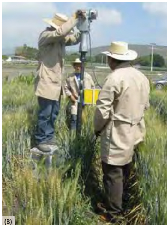
Figure 17.1. Soil coring using: (A) a tractor with 'Giddings' hydraulic soil corer; and, (B) a hand-held soil corer.
