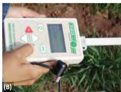
Figure 11.1. Taking light interception measurements with a hand-held ceptometer: (A) measurements below the spike; (B) the Decagon AccuPAR LP-80 ceptometer; and, (C) measurements at GS31, also showing the external sensor being held for simultaneous above-canopy measurements.
