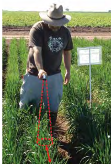
Figure 1.6. Shows the use of the IRT during in-field measurements at the pre-heading phase on bed plots with two rows. The dotted red lines illustrate the field of view of the IRT, and the arrow illustrates movement of IRT out and back over the crop (remembering to avoid the ends of the row which act as the border).
