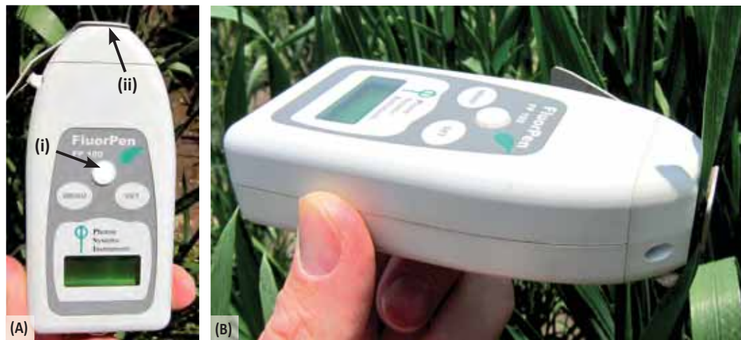
Figure 13.2. Hand held chlorophyll fluorometer Fluorpen FP-100: (A) showing (i) PAR sensor, and (ii) sample leaf in sensor chamber; (B) field measurements in daylight conditions.
