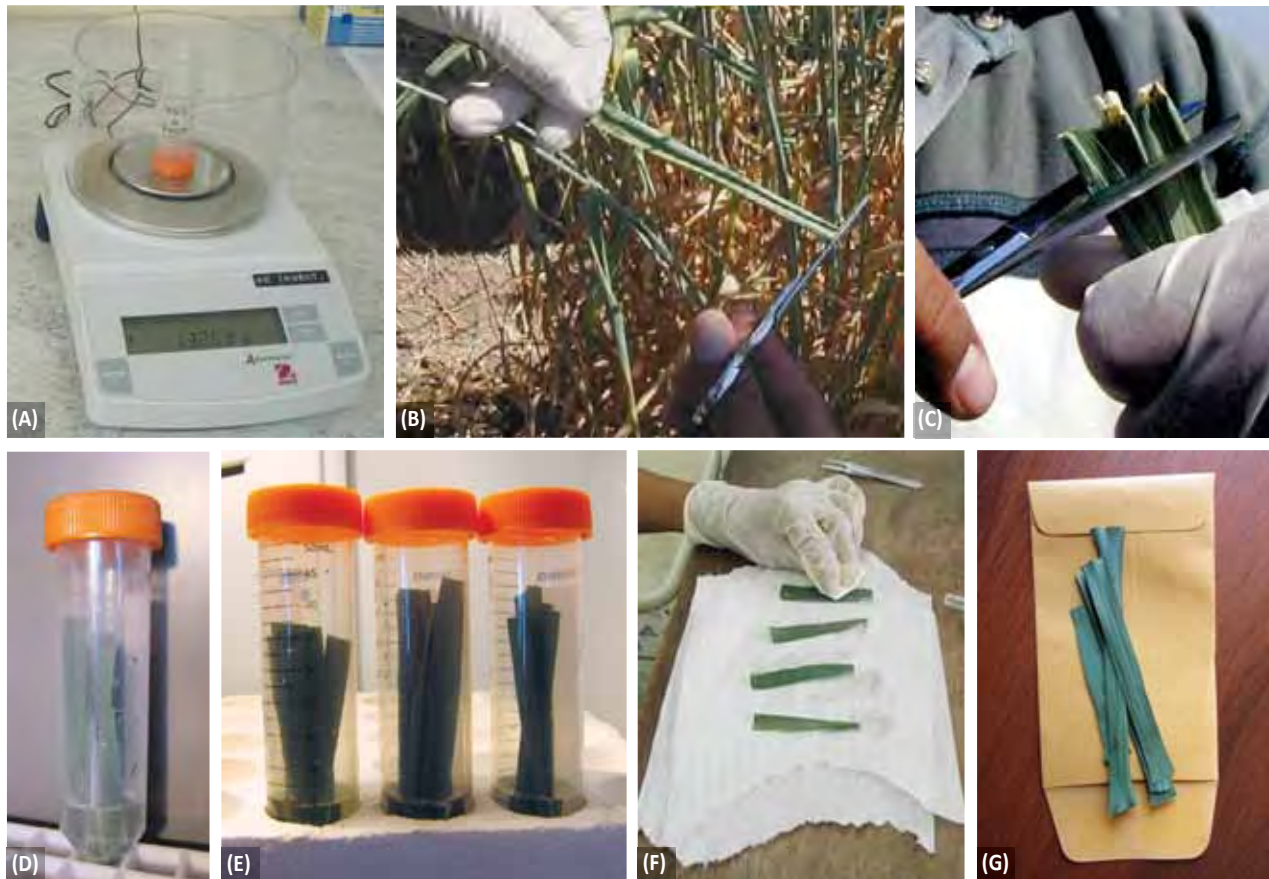
Figure 5.1. Measuring the leaf relative water content: (A) weighing empty tubes; (B) select and cut leaves in the field; (C) cut the top and bottom of all leaves together; (D) tube containing leaf samples filled with 1 cm of distilled water; (E) sample tubes in the refrigerator; (F) carefully blot dry the turgid leaf samples; and, (G) dried leaf samples.
