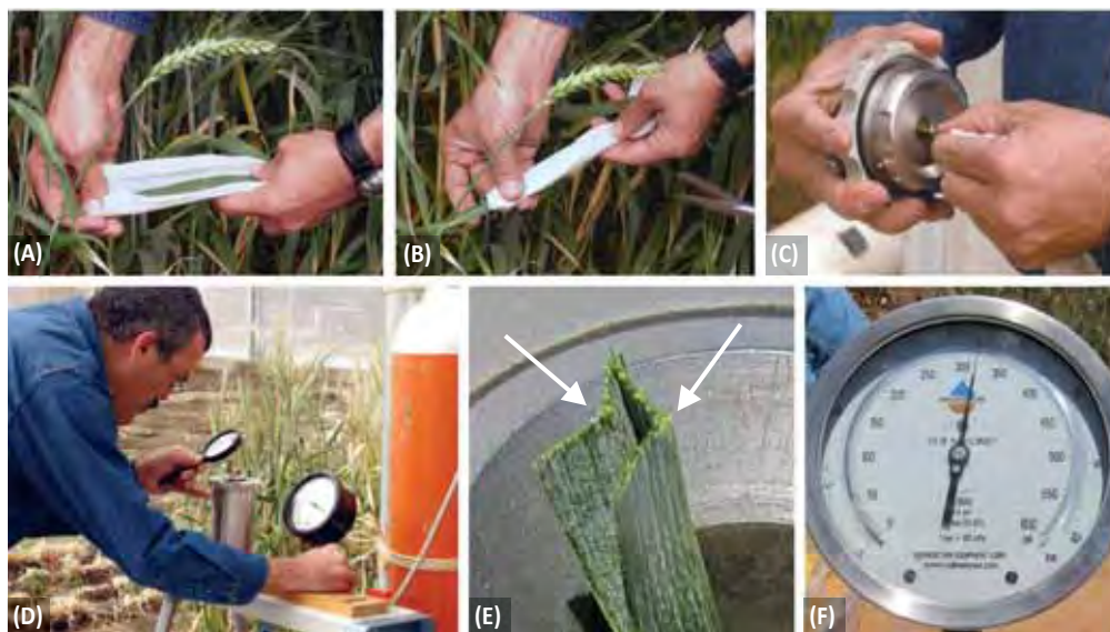
Figure 3.2: Leaf sampling and leaf water potential measurement: (A) first wrap the selected flag leaf in a moist gauze; (B) and then cut the leaf at the base; (C) place the leaf sample within the rubber seal of the top of the pressure chamber; (D) use a magnifying glass to observe the point at which water appears at the cut ends; (E) water exuded from the vascular tissue; and, (F) the reading on the pressure dial (22 bar).
