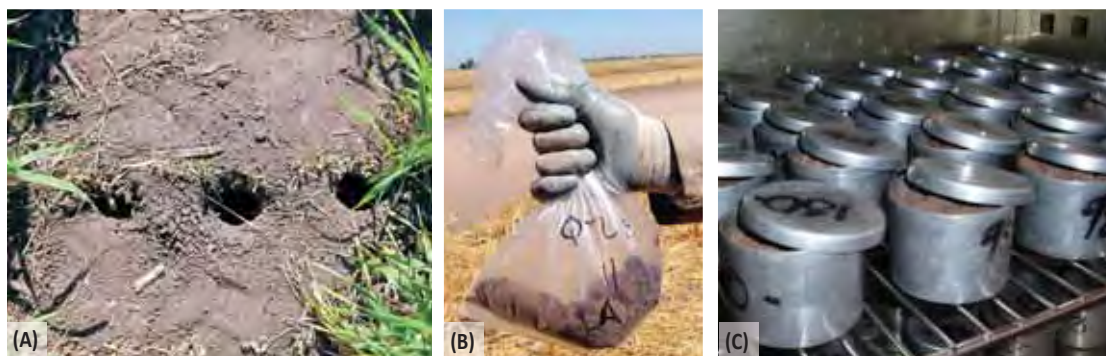
Figure 17.2. Soil coring: (A) coring in the biomass cut with multiple samples per plot; (B) soil core sample in labeled plastic bag; and, (C) soil sub-samples drying (lids slightly ajar to allow moisture to evaporate).
