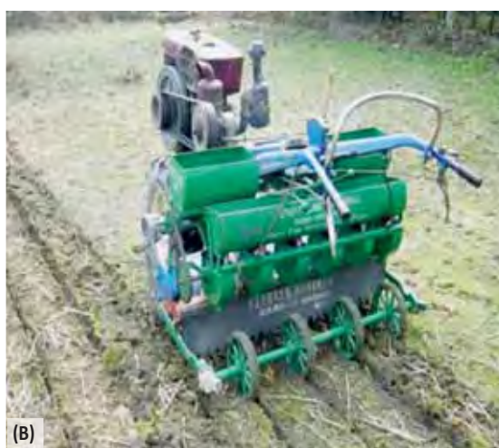
Figure 15.7. Use of CA-based seeders with 2-wheel tractors in Bangladesh for (A) strip till seeding of wheat after rice, and (B) zero till seeding of chickpea.
