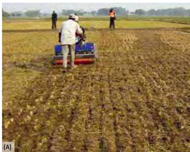
Figure 15.7. Use of CA-based seeders with 2-wheel tractors in Bangladesh for (A) strip till seeding of wheat after rice, and (B) zero till seeding of chickpea.
