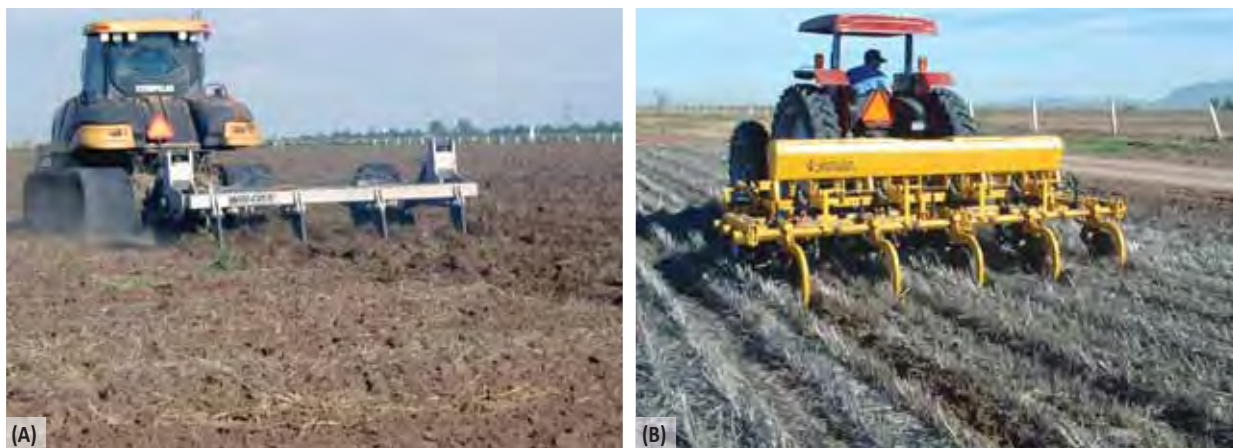
Figure 15.1. (A) Conventional till system versus (B) permanent raised bed system.
